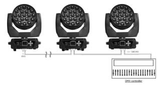
Connect the DMX-output of the first fixture in the DMX-chain with the DMX-input of the next fixture.
